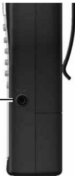
**PC/IF** — connect an optional PC interface cable here to use the scanner with your computer.
