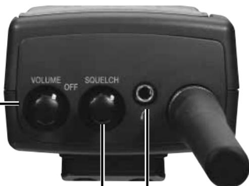
**VOLUME** — turn the scanner on or off and adjust the volume.
