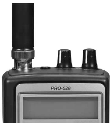
When using an external antenna, always use 50-ohm, RG-58, or RG-8, coaxial cable to connect to it. If the antenna is over 50 feet from the scanner, use RG-8 low-loss dielectric coaxial cable. If your antenna's cable does not have a BNC connector, your local RadioShack store carries a variety of BNC adapters.
