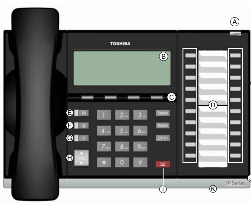
**20 Programmable Feature Buttons 4-Line LCD Telephone**
