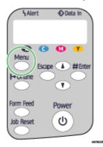
2. Press [▲] or [▼] key to display [System], and then press the [#Enter] key.
