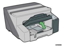
2. Hold the Tray 1 grip, pull the tray halfway out, lift it slightly, and then pull it out further.
