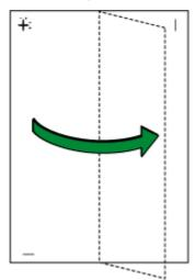
9. The optimal adjustment value is the difference between the single vertical line and the cross's vertical line that you can see when the folded paper is held up to light. When the difference is one calibration mark in the "+" direction, the optimal adjustment value for the [Read Direction] is "+1.0".
