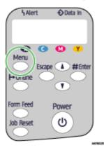
2. Press the [▲] or [▼] key to display [Host Interface], and then press the [#Enter] key.
