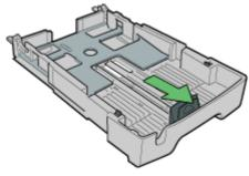
5. Slide the tabs back into place to lock the paper tray extension into position.
