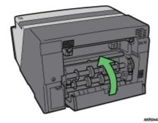
Check that the duplex unit is correctly attached and the duplex unit cover is closed.
