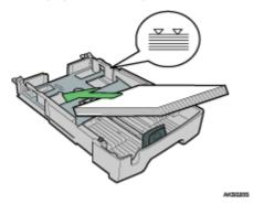
8. Squeeze the front end paper guide, and then slide it to meet the edge of the paper.
