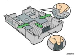
Beforehand, make sure to squeeze the front end paper guide, and then expand the guide.
