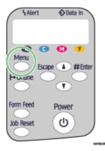
2. Press the [▼] or [▲] key to display [Maintenance], and then press the [#Enter] key.
