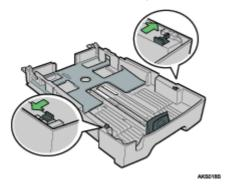
6. Squeeze the paper guide release, and then slide the paper guides into position according to the paper size.
