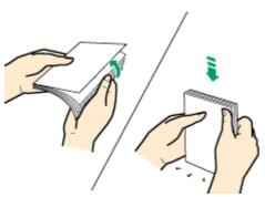
Before loading envelopes, make sure their edges are sharply creased by rubbing the edges with a pen or similar object.
