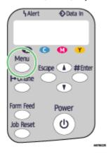
3. Press the [▼] or [▲] key to display [Maintenance], and then press the [#Enter] key.
