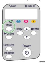
2. Press [▲] or [▼] to scroll to "Paper Input" on the display, and then press the [#Enter] key.
