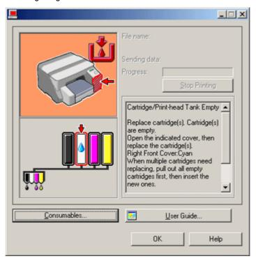
• In this illustration, the cyan Print cartridge has completely run out.
