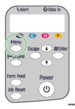
2. Press the [▼] or [▲] key to display [List/Test Print], and then press the [#Enter] key.
