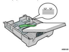
5. Squeeze the front end paper guide, and then slide it to meet the edge of the paper.
