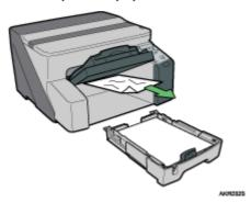
If you cannot remove the jammed paper or it is difficult to remove, the paper may be jammed inside the printer. Examine the paper carefully and remove.
