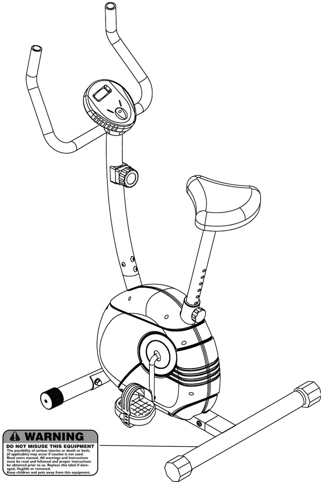
The Warning Label shown here has been placed on the Rear Stabilizer. If the label is missing or illegible, please call customer service at 1-800-999-8899 for replacement. Apply the label in location shown.
