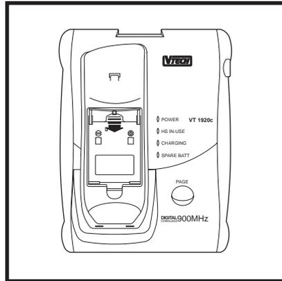
Place a battery pack in the Spare Battery charger. Make sure the metal charging contacts on the underside of the battery pack are aligned with the charging contacts in the Spare Battery charger.
