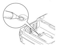
2 Install 2 AA batteries, matching the polarity symbols (+ -).
