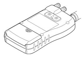
Warning: Set ALKALINE/RECHARGEABLE to RECHARGEABLE for use only with nickel cadmium (Ni-Cd) or nickel metal hydride (Ni-MH) rechargeable batteries. Never attempt to recharge non-rechargeable batteries. Non-rechargeable batteries can get hot or explode if you try to recharge them.
