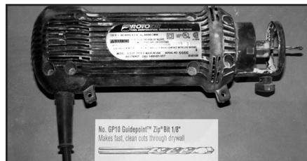
Fig. 11: Rotozip™ showing guidepoint bit.
