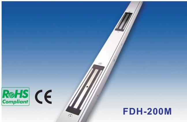
FDH electromagnetic lock has been designed to embed the electromagnet in the doorpost and it offers to 600 LBS holding force. The doorpost is installed horizontally on the header of the door-frame. Hence, the doorpost and doorframe will be shaped into one and provides superior appearance.
