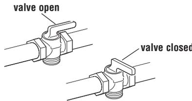
**3.** Open shutoff valve in the gas supply line. The valve is open when the handle is parallel to the gas pipe.
