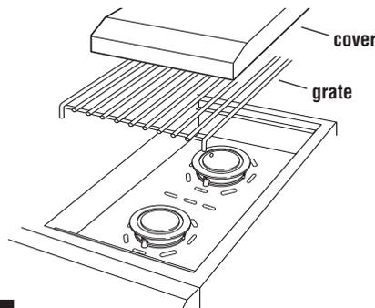
**5.** Carefully lift off cover and grate and set aside. Remove packing from around burners. Reinstall grate.
