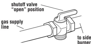
The supply line shall be equipped with an approved shutoff valve. This valve should be located in the same area as the side burner and should be in a location that allows ease of opening and closing. Do not block access to the shutoff valve. The valve is for turning on or shutting off gas to the appliance.
