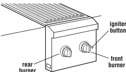
2. Push in the burner igniter button. You will hear the "snapping" sound of the spark. Keep the burner igniter button pushed in until burner lights. Make sure burner is lit. Repeat for the other burner as needed.
