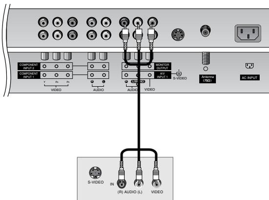
The TV has a special signal output capability which allows you to hook up a second TV or monitor.
