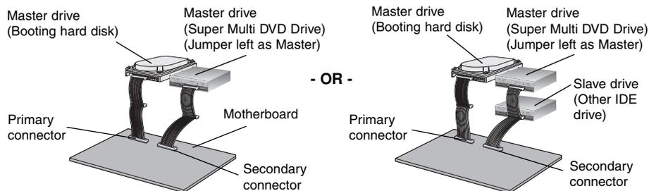
**NOTE :** A hard disk is normally installed as the Primary Master on the EIDE (ATAPI) interface. Other EIDE peripheral devices such as hard drives and Super Multi DVD Drives are then set differently.
