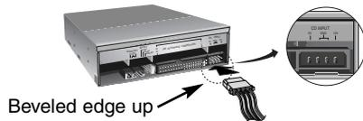
**NOTE :** Improper connection may damage the drive and void the warranty. Generally, the power connector can only fit one way.
