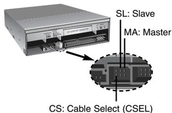
**NOTE** : If two peripheral devices with the same settings are both connected to the Primary or to the Secondary EIDE bus, the host computer may fail to run or may malfunction. Careful attention is necessary.
