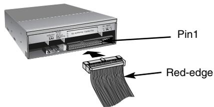
**NOTE :** Generally, the IDE connector is keyed and will only fit one way.
