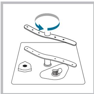
Food residue may become encrusted onto the sprayer arms and block the holes used to spray the water. It is therefore recommended that the arms are checked from time to time and cleaned with a small non-metallic brush.
