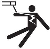
• **ELECTRIC SHOCK CAN KILL.** Unless using COLD FEED feature, when feeding with gun trigger, the electrode and drive mechanism are always electrically energized and could remain energized several seconds after the welding ceases..
