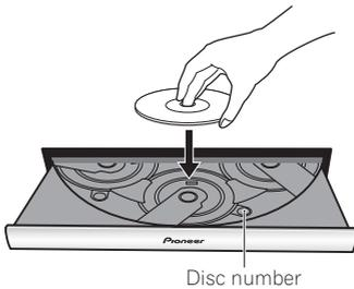
If you want to load more discs, press **DISC SKIP** (remote or front panel) to rotate the disc tray. You can load up to five discs at once.
