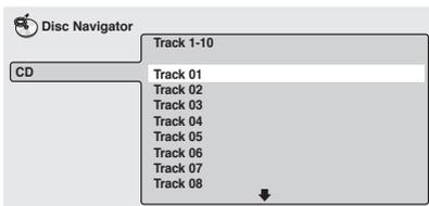
The screen for WMA/MP3 discs shows the folder names on the left and the track names on the right (note that any folder and track names that contain accented or non-roman characters, will show up with generic names – **F\_033**, **T\_035**, etc.).
