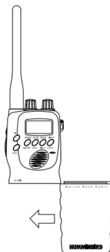
Install four new batteries in each half of the battery pack. Assure the positive and negative orientation of the batteries match the engraving on the inside of the battery back. To reassemble the battery pack, first mate the two halves together at the bottom and then snap shut. Slide the battery pack onto the radio. When the battery is low, a battery icon appears on the LCD. The battery pack can be charged on or off the VHF5 unit.
