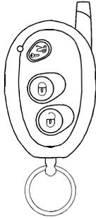
1. The Lock button on the transmitter is used to lock the vehicle's doors, the Unlock button is used to unlock the vehicle's doors. To lock or unlock the doors simply press and release the desired function button one time. As a keyless entry unit, for your convenience, the parking lights will flash once when the doors are locked and twice when the door are unlocked.
