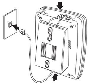
5. Plug one end of the telephone cord into the **TEL LINE** jack on the back of the base. Plug the other end into a telephone jack.
