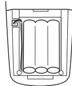
4. Slide the battery cover forward until it snaps into place
