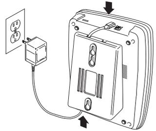
4. Put the AC adaptor cord inside the wall mount adaptor. Plug the AC adaptor into a standard 240V AC wall outlet.
