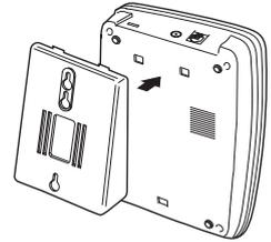
3. Plug the AC adaptor cord into the 9V DC input jack on the back of the base.
