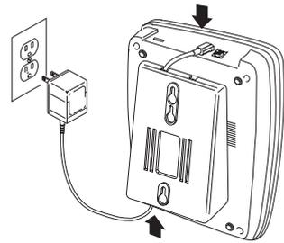
5. Plug one end of the short telephone cord (not supplied) into the **TEL LINE** jack on the back of the base. Plug the other end into a standard telephone jack, through wall mount adaptor hole.
