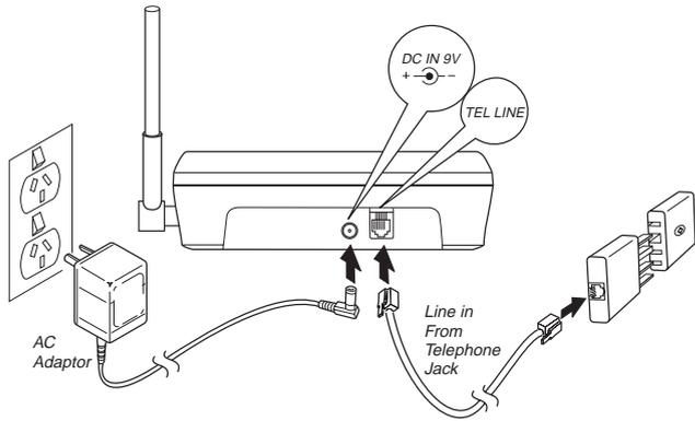
1. Plug the AC adaptor cord into the **9V DC** input jack on the back of the base.
