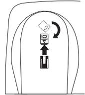
8. Flip the retainer from front to back. Slide it back into the slot so that the lip of the retainer is up (arrow on the retainer clip must be pointing down). The retainer holds the handset in place.
