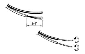
3. Insert about 1/2-inch of the wire that you have identified as positive into the red (+) connector on your right-channel speaker. Insert the other end of this positive lead into the RIGHT (red) Speaker 1 terminal on the back of your amplifier. Tighten the terminal knob, and the wire will be held securely.
