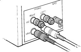
The other set of jacks is marked MM, for Moving Magnet. If you have a regular moving magnet cartridge mounted on your turntable, connect the turntable only to the MM inputs, as the sizeable volume boost of the MC jacks will cause volume problems and severe distortion.
