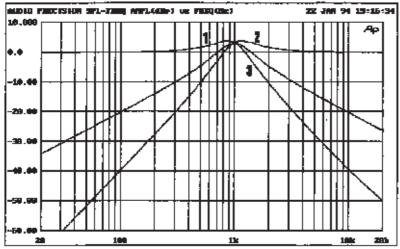
of the audio spectrum to contrive a bandpass filter for the production of 'telephone' effects and similar treatments.
