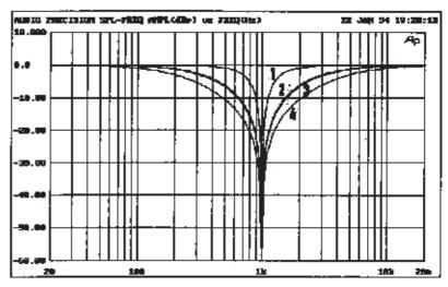
a notch across the audio spectrum. A further creative use is to create a pseudo stereo image from a mono signal by splitting the signal and applying different notches to each of the two channels. If these two channels are then panned left and right in the final mix, it creates an illusion of space. The position, number and width of the notches must be fine tuned by ear.
