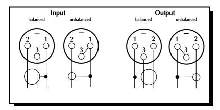
pin 3 cold). Unbalanced inputs and outputs are also available on mono, quarter-inch jacks.
