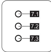
After having pressed the button **5** the light **7.1** (Wash) and **7.2** (Door) illuminate to indicate that appliance is working and the door is locked.
