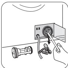
Remove any objects from the pump impeller by rotating it. Put the cap back on the emergency emptying hose and place the latter back in its seat.
