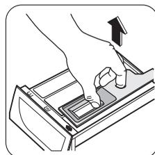
To aid cleaning, the top part of the additive compartment should be removed.
