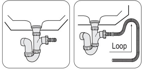
If the outlet spigot has not been used before, remove any blanking plug that may be in place.
