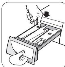
Remove the drawer by pressing the catch downwards and by pulling it out. Flush it out under a tap, to remove any traces of accumulated powder.
