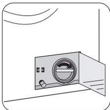
Screw the pump cover fully in. Close the pump door.
