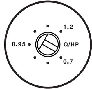
Setting the “Q” is a subtle process. It is recommended that the “Q” setting be left in the 0.7 position and adjusted only after the input sensitivity and highpass crossover ranges are known. Small adjustments to the “Q” setting are all that are required to fine-tune the system.
