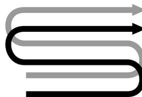
Figure 10: Use an overlap technique on every pass.
