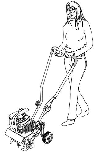
Figure 9: Assume operator's position once engine starts.
