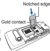
5. Place the SIM card holder back in place and slide in the direction of the “Lock” arrow to secure.
