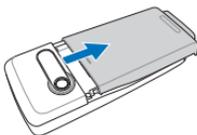
2. Remove the battery. The battery compartment has a groove at the top to make it easier to remove the battery.
