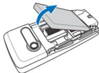
3. Push the SIM card holder in the direction of the “Open” arrow, then lift it using your fingernail.
