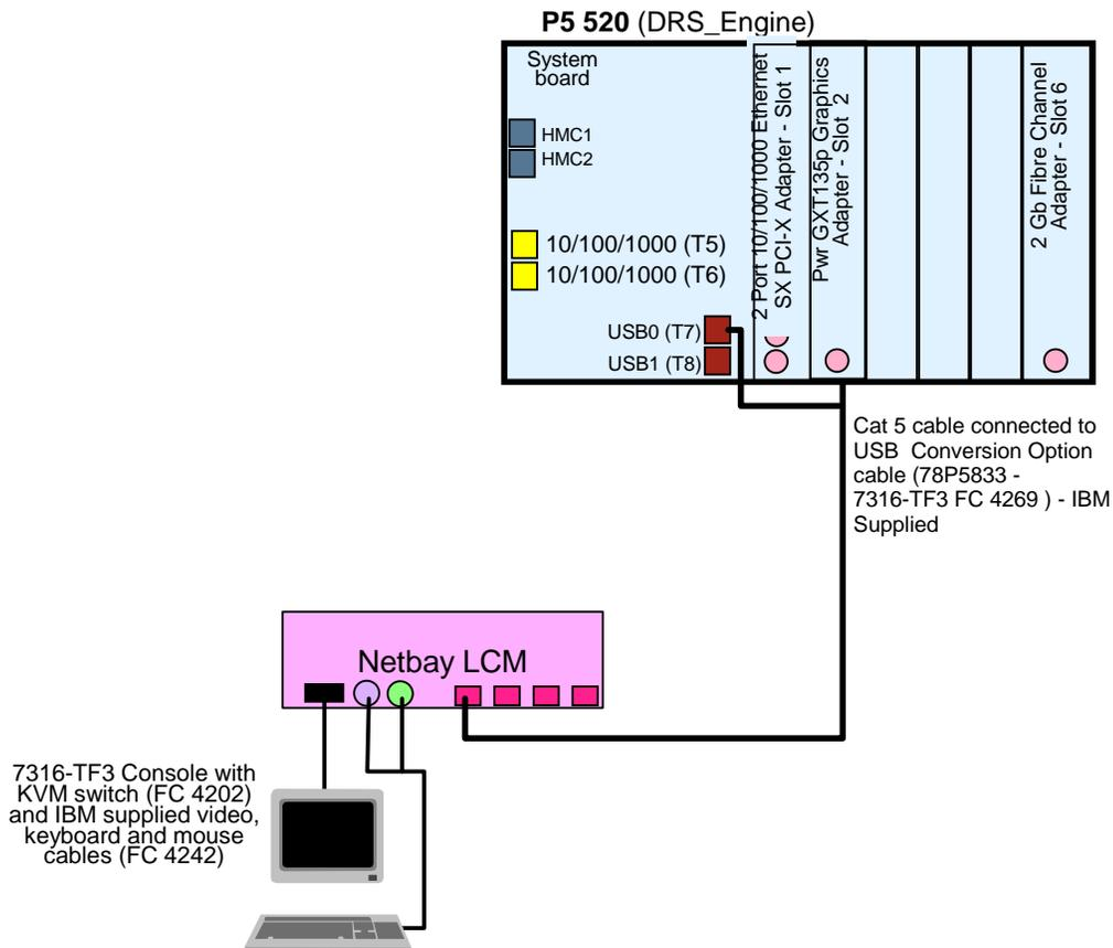
As an option, you can attach an external monitor using the serial port on the P5 520. To interact with the system software interfaces or to run diagnostics from a DVD-RAM using an external device, you will need to do the following:
