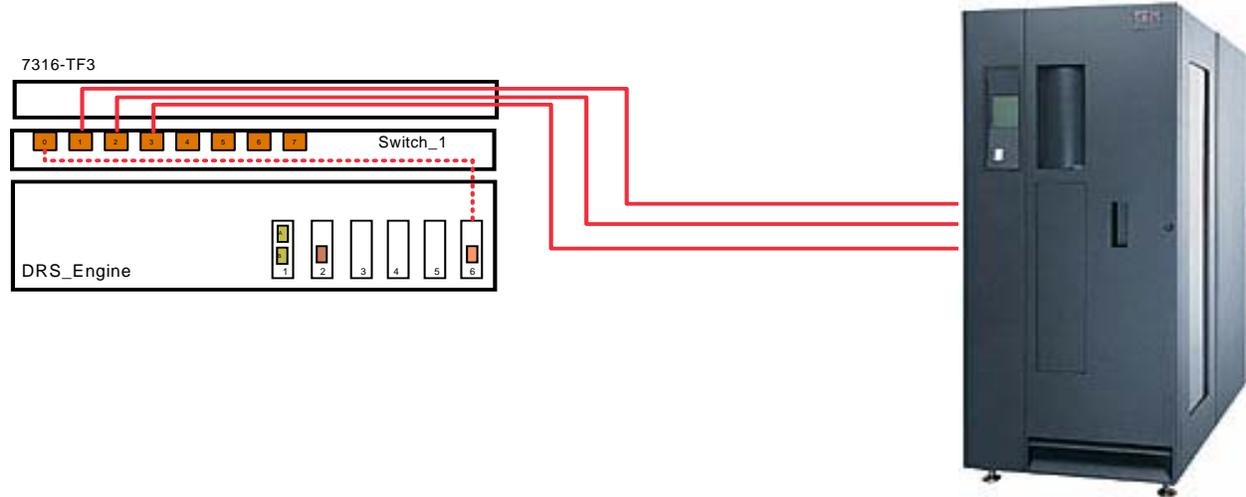
In the diagram above, the orange (dotted) cables represent the connections between the HBAs in the servers and the ports on the SAN switches. The solid lines (orange) represent connections to the tape drives. You will use switch ports 1-3 for tape connections. You can have up to three 3592s attached in this configuration.
