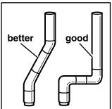
exhaust vent. Use the fewest number of elbows and turns. Allow room when using elbows or making turns. Bend vent gradually to avoid kinking.
