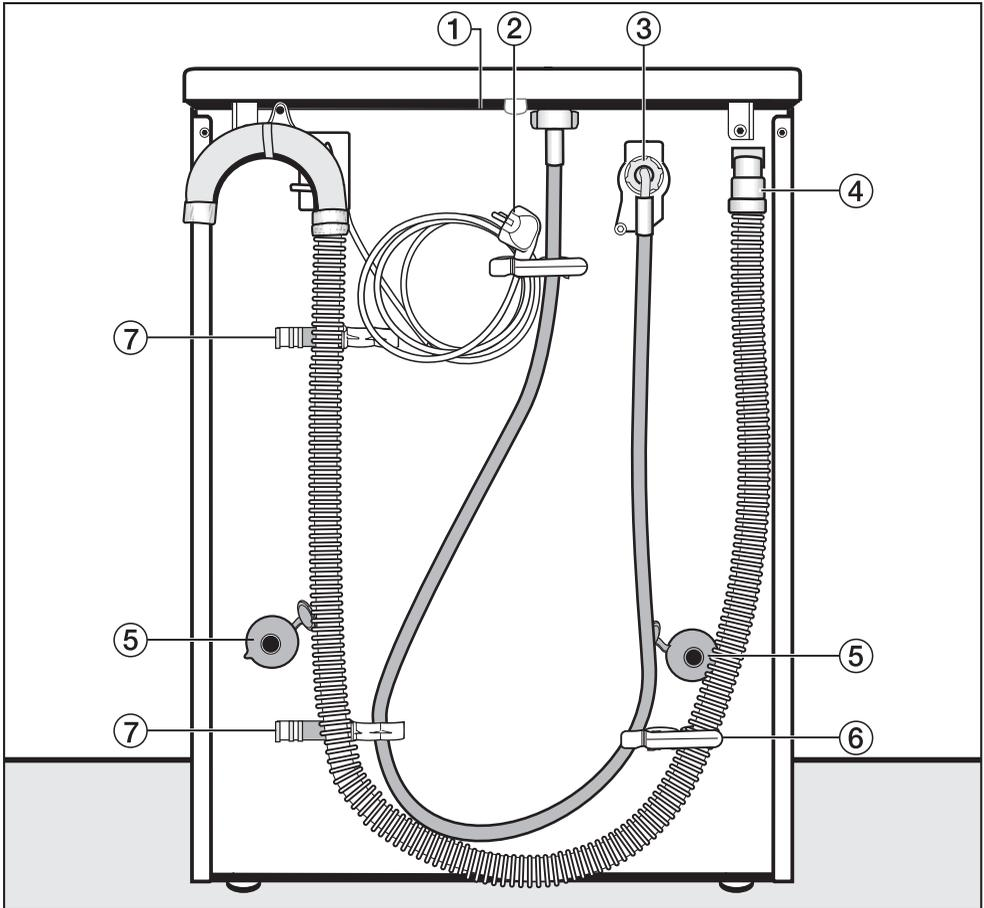
① Protruding lid for holding when moving the machine
