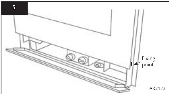
There are two fixing brackets either side of the controls:
