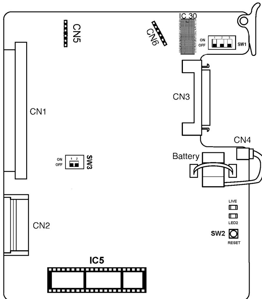
**Figure 2-2: CPUI( )-U( ) ETU Switch Settings**
