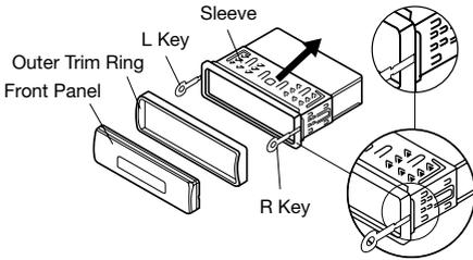
6. Mount the sleeve by inserting the sleeve into the opening of the dashboard and bend open the tabs located around the sleeve with a screwdriver. Not all tabs will be able to make contact, so examine which ones will be most effective. Bending open the appropriate tabs behind the dashboard to secure the sleeve in place.
