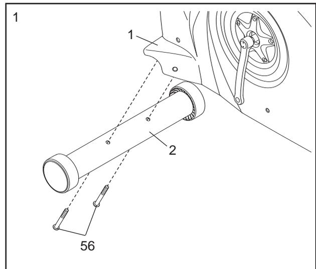
2. Attach the Rear Stabilizer (3) to the Frame (1) with two M10 x 85mm Button Screws (56).
