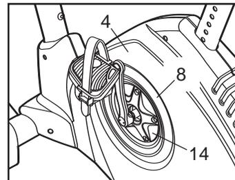
Next, locate the Reed Switch (49). Turn the Left Crank Arm (15) until the Magnet (23) is aligned with the Reed Switch. Loosen, but do not remove, the indicated M4 x 16mm Screw (54).
