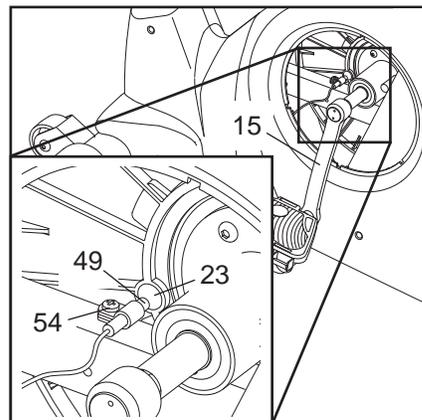
Slide the Reed Switch slightly closer to or away from the Magnet. Then, retighten the Screw. Turn the Left Crank Arm for a moment. Repeat until the console displays correct feedback. When the Reed Switch is correctly adjusted, reattach the left Pedal Guard (8) and the left Side Shield Cover (14).
