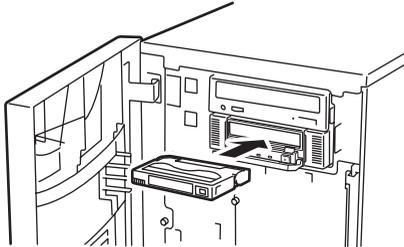
By fully inserting the data cartridge, it is automatically set in the drive and the TAPE MOTION LED lights.
