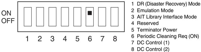
When switch 6 is ON, cleaning requests are enabled. When enabled, the “CLEANING REQUEST” LED on the front panel lights after every 100 hours of operation.
