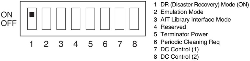
\* In Disaster Recovery Mode, an SDX-800V series drive enters the DR Standby Mode 15 seconds after you insert a write-protected tape into the drive, and all the drive LED blink. If you restart the drive while the LED are blinking, it starts as a CD-ROM device.
