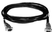
**TAXI:** The standard 25' (7.6 m) cable (6050-0148-CE) has DB-9 Male connectors with screw-down locking hardware. The TAXI (Serial communication) cable interconnects the "Serial Com" connector on the rear of the ST-133 with the PCI card installed in the host computer. In addition to the standard length, this cable is available in 10', 50', 100', and 165' lengths. Also available are fiber optic adapters with fiber optic cables in 100, 300, and 1000 meter lengths.
