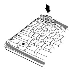
When you wrap the cord around each post, gently pull some of the slack out of the cord so that it does not sag too much over the side of the keyboard and so that the connector reaches well into the nesting area. For proper sliding action, nest the connector as close to the far left side of the nesting area as possible.
