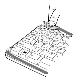
Next, unwind the cord from the two posts on the right side of the keyboard and then from the post on the bottom left side.
