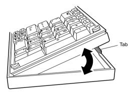
The top cover has footpads on it, so no matter whether you use the keyboard flat or in the tilt position, it should not slide on your work surface.
