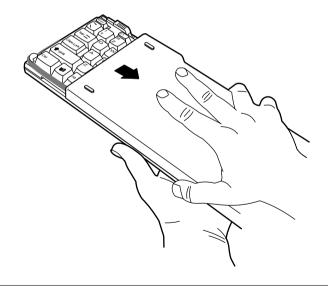
Next, put the keyboard flat on your work surface and pull the connector out of its nesting area.
