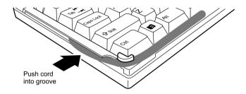
After you have put the cord in this stored position, it is easiest to put the cover back on the keyboard by following this procedure:
