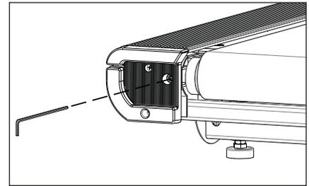
**Note:** Do not exceed one full turn of the adjusting screws in either direction. If after one full turn the belt does not track properly, contact Customer Support Services.
