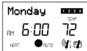
Step 3 The Program hour and AM or PM indicator are flashing. Press
