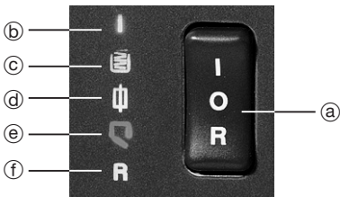
Bedienfeld ④ IDEAL 4000/IDEAL 4003 Control panel ④ IDEAL 4000/IDEAL 4003 Panneau de commande ④ IDEAL 4000/4003
