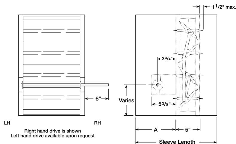
The standard location of a damper mounted in a factory sleeve ("A" dimension) is shown below. The damper can be positioned at other locations within a range of 6 in. (152 mm) to 12 in. (305mm) for the "A" dimension.
