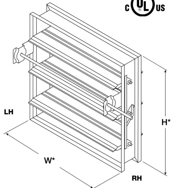
\*W&H dimensions furnished approximately 1/4 in. (6 mm) undersize. (Add sleeve thickness for overall sleeved damper dimension)
