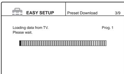
If the Preset Download function does not work or if you made a connection other than **A** (page 17), the Auto Tuner Preset function automatically starts searching for all of the receivable channels and presets them.
