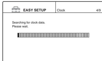
If the current time or date is not set, “The clock was not set automatically. Set the time and date manually.” appears. Set the clock manually using ←/↑/↓/→, and then press ENTER.
