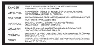
This label is located on the laser protective housing inside the enclosure.
