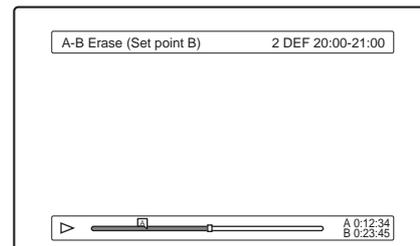
**5 While watching the playback picture, set point B using ▷, ||, and ◀/▶, then press ENTER.**
