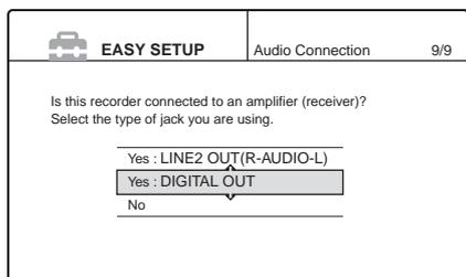
**19 Press ↑/↓ to select the type of jack (if any) you are using to connect to an amplifier (receiver), then press ENTER.**
