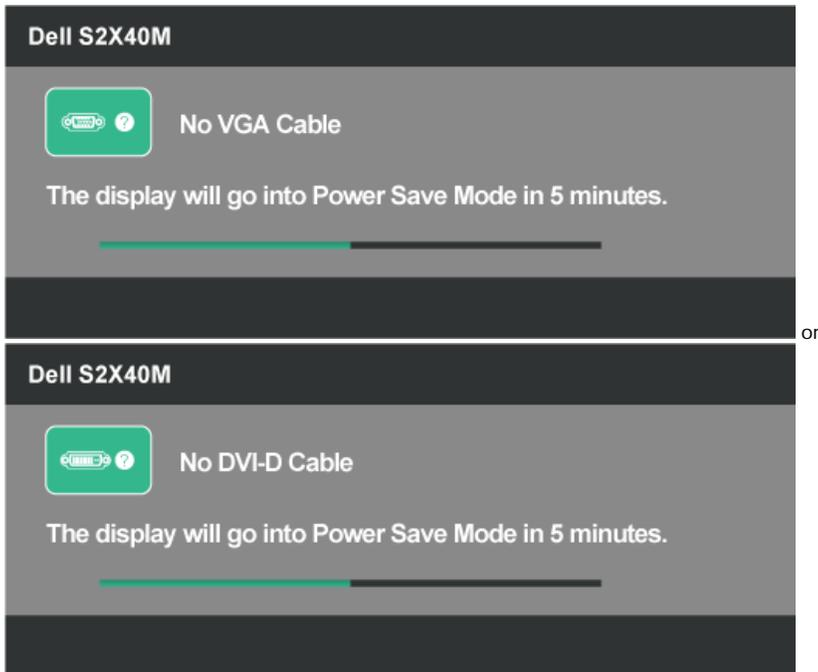
4. This box also appears during normal system operation, if the video cable becomes disconnected or damaged. The monitor will enter **Power Save Mode in 5 minutes** if left at this state.
