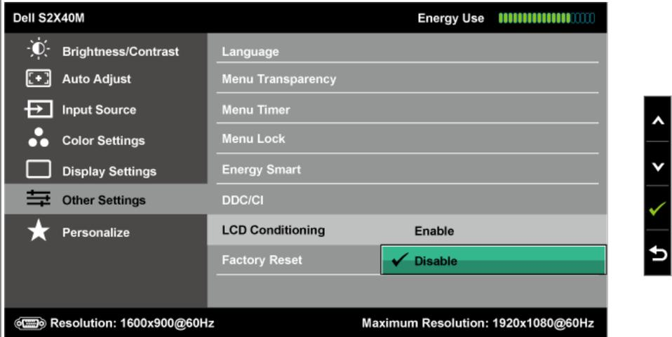
If an image appears to be stuck on the monitor, select **LCD Conditioning** to help eliminate any image retention. Using the LCD Conditioning feature may take some time. LCD Conditioning feature cannot remove severe cases of image retention or burn-in. **NOTE:** Use LCD Conditioning only when you experience a problem with image retention.
