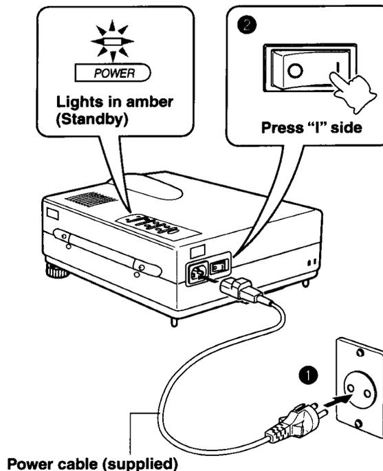
**2) Press the POWER ON button on the remote control or the POWER button on top of the unit to turn on the unit.**
