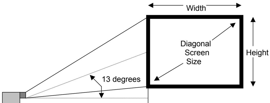
Use the following information to position the projector. Horizontally the projector needs to be positioned with the lens-centered left to right
