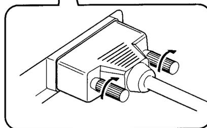
**Plug the cable terminal into the RGB connector securely then tighten the screws.**
