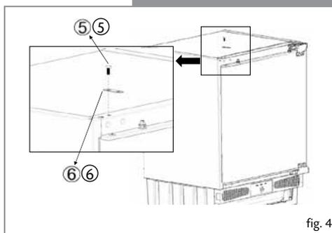
**Fig. 5 - Fitting the spacer piece**
