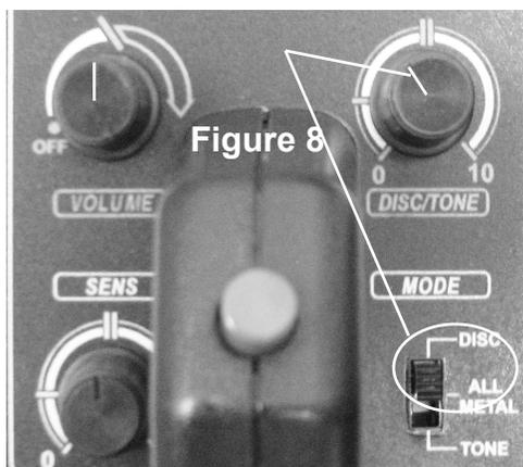
Sweep the nickel in front of the Search Coil; the unit will not respond to the nickel or to the iron nail. But it will respond the other samples.
