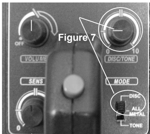
3. As a test, sweep the iron nail sample 2 to 3 inches above the search coil. The unit will NOT respond (the meter pointer won't swing and the unit is silent.) Sweeping the other samples should produce the “DI” tone and make the pointer move.
