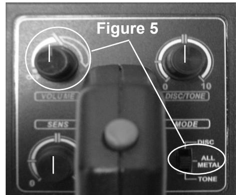
Sweep the metal samples 2 to 3 inches or more above the center of the Search Coil. The Metal Detector will respond to each with a “DI” tone and the pointer on the View Meter will swing to the right.
