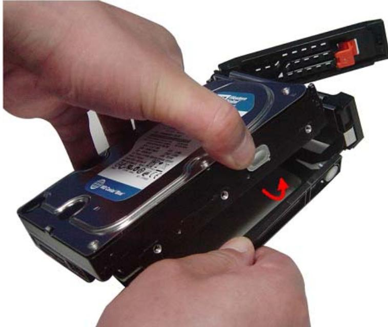
4. Remove the removable HDD bracket.
