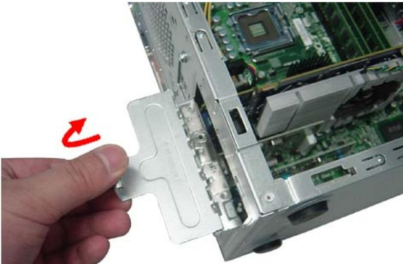
3. Use a finger to press the clip, and the same time Gently pull the card to remove it from the mainboard.
