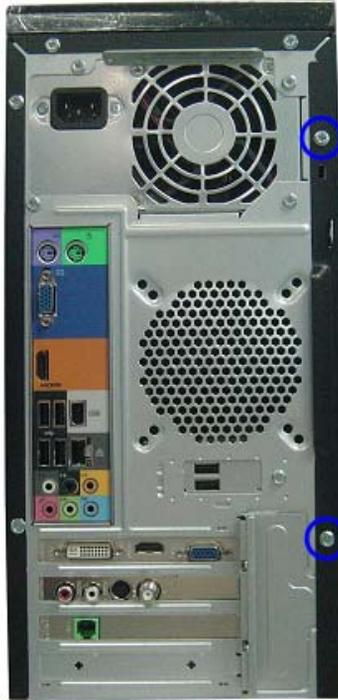
2. Slide the side panel toward the back of the chassis until the tabs on the cover disengage with the slots on the chassis.
