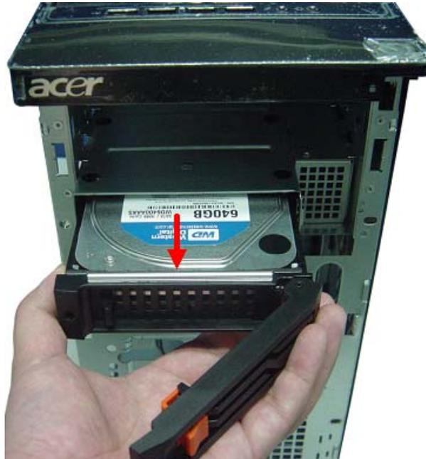
3. Remove the HDD module
