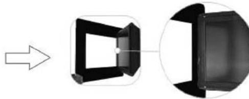
3. To reattach a new frame, simply hold the back cover at a slight angle, then insert the two wedges on the other side of the back cover into the matching holding slots of the frame. Gently lower the back cover while pressing on the latch until it clicks onto the frame.
