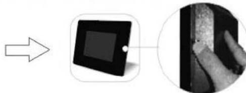
2. Lift the back cover and gently pull it from the two holding slots on the other side of the frame.
