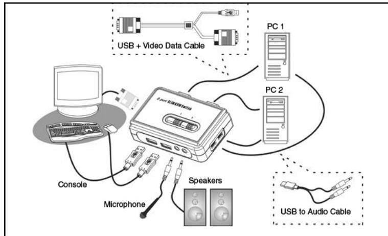
2. Using a USB + Video Data Cable, connect one end (blue) to the video out connector on **computer 1**. (This will be the same connector from which you disconnected the monitor in step 1, if applicable.) Connect the opposite end to the VGA port on the back of the KVM Switch.
