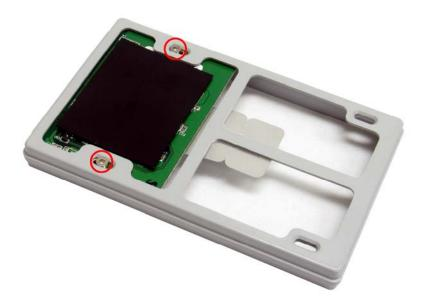
Caution: Be sure to remove the circuit board from the plastic holder before attaching the hard drive; otherwise, the hard drive's IDE pins may be damaged.
