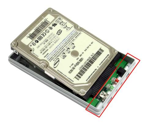
**Step 7** Turn the plastic holder over. Use the provided screws and the screws removed in Step 4 to secure the hard drive onto the holder.
