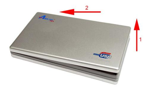
**Step 3** Remove the bottom cover in the same manner. If you find it hard to lift the plastic holder, press it slightly inward.
