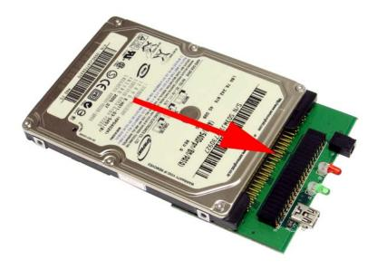
**Step 6** Replace the circuit board and the hard drive back to the plastic holder. Verify that the connectors and LED indicators are properly aligned with the openings of the holder.
