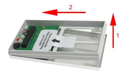
**Step 4** Unscrew the two screws that hold the circuit board and remove it from the plastic holder. Remove the sticker that is on the circuit board as well.
