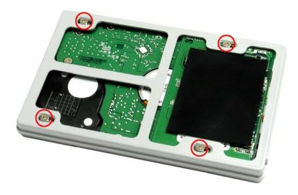
**Step 8** Replace the bottom cover to the holder and then replace the upper cover. Be sure to hook the latches when replacing the covers.
