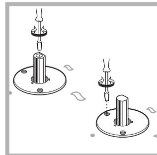
2. Remove the knob and turn the regulator screw (positioned either on the side of the top or inside the shaft) clockwise until the flame becomes small but regular.
