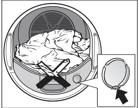
If you are not using a fragrance flacon: the tab must be pushed down completely (see arrow).
