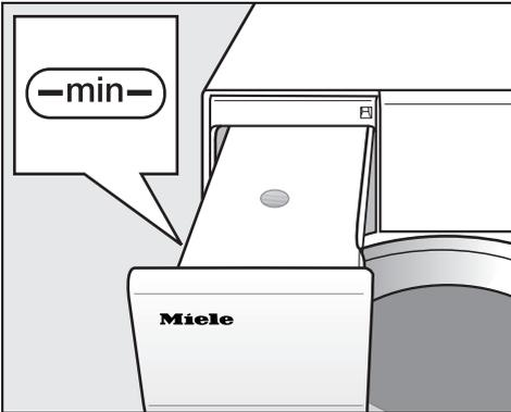
The **-min-** marker is at the front left-hand side of the container.
