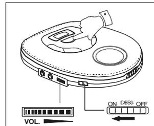
6. Adjust the VOLUME and DBBS (Bass Boost) controls as desired.
