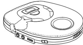
To search forward or backward within a track to locate a specific musical passage press and hold either the SKIP FWD **▶▶** or SKIP REV **◀◀** buttons. The player moves forward or backward at high speed. When you reach the desired point in the track, release the buttons and normal playback resumes.
