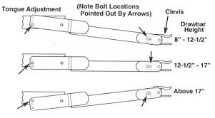
It is important that the MP and FP are both operated in a level position. Leveling can be accomplished by adjusting the tractor draw bar height, also by leveling the mower frame by use of the adjustable jack stand.
